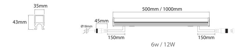
Tolerance for dimensions =  $\pm 2.5$ mm
